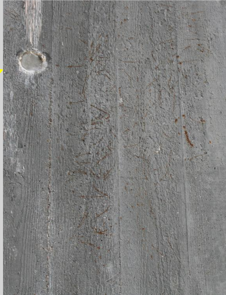
Figure 8.24: Transition zone from SFRSCC in the walls to SFRC in the deck (black dotted line). Visible fibres within the yellow ellipse.
