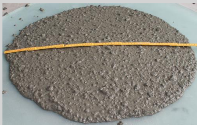
Figure 1.2: Top: Slump of traditional concrete. Bottom: Slump flow of self-compacting concrete.
