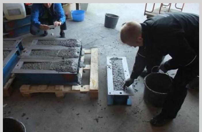
Careful manual finishing to level the surface.
