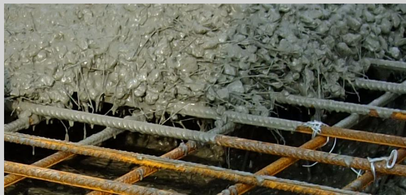
Figure 2.3: Example of fibre blocking on top of a reinforcement mesh.
