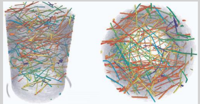
Figure 5.10: Concrete core sample scanned by computed tomography and analyzed by image analysis [Fritz2009].
