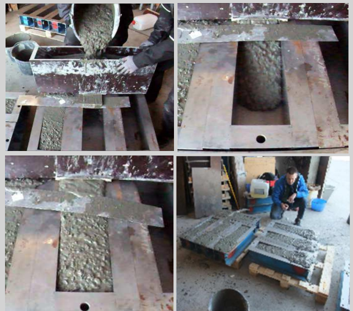
Figure 7.18: Casting of 18 standard beams.
