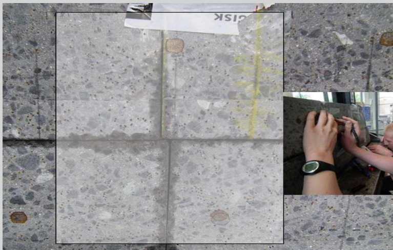
Figure 7.39: Cut columns split into smaller samples. Manual fibre counting at the right.
