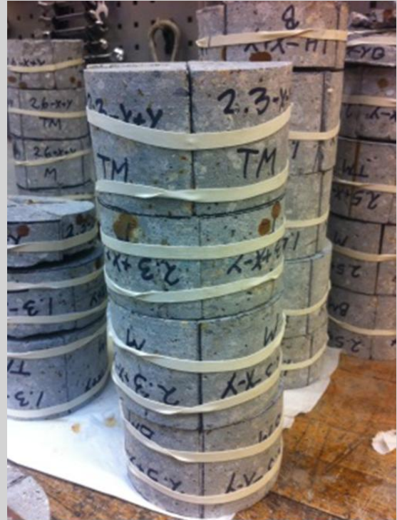
Figure 7.61: Example of a drilled core split into different sections.
