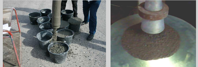
Figure 7.17: Left: Sampling after pump. Right: Measurement of the rheological properties using the 4C-Rheometer.
