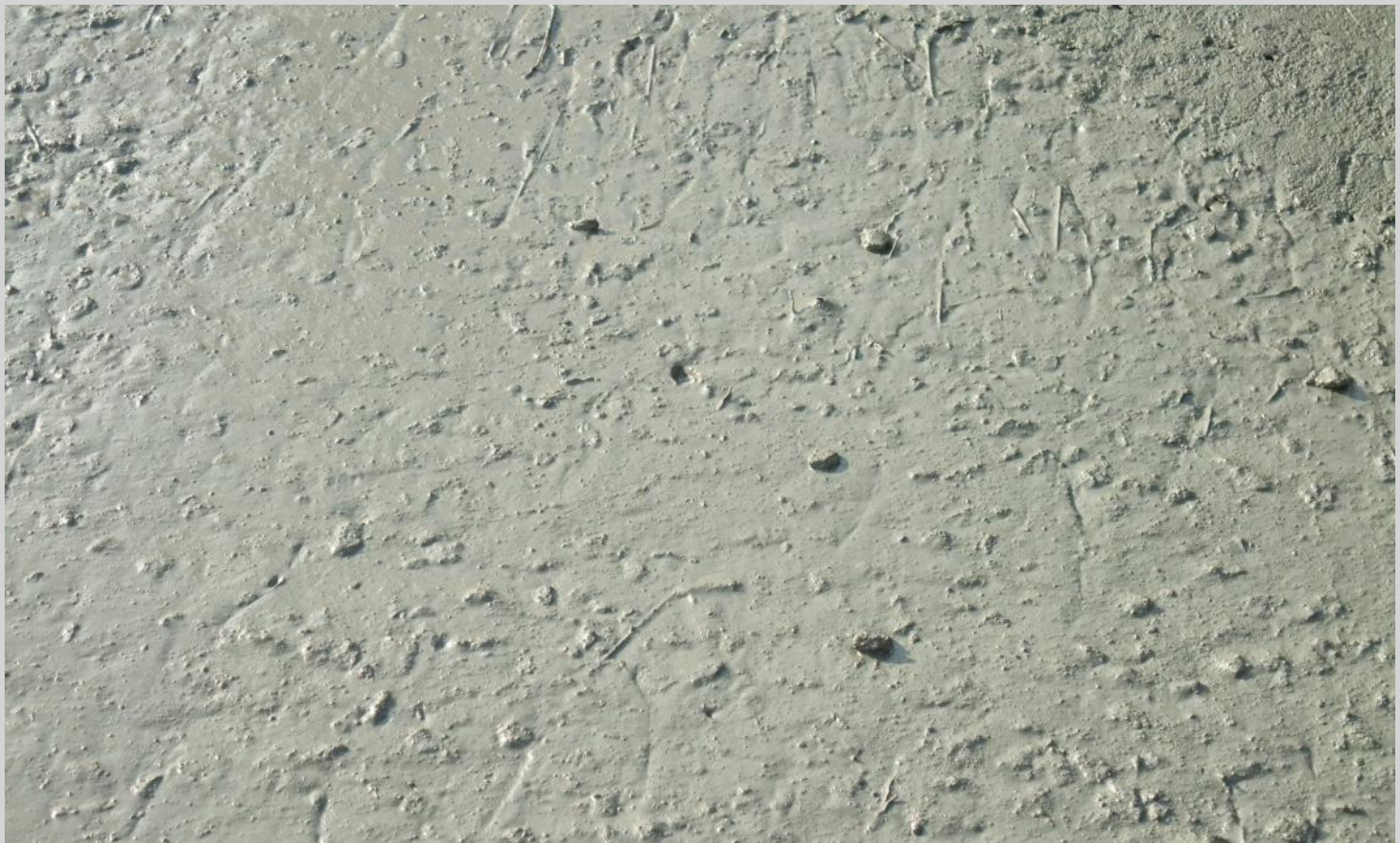
Figure 8.13. The surface appearance after applying a beam vibrator on top of conventional SFRC.
