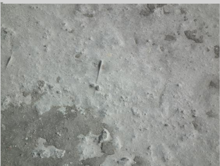
Figure 8.11. The surface appearance of SFRSCC after manual trowelling. No other surface finishing procedures have been applied. Difficult to submerge all the fibres.
