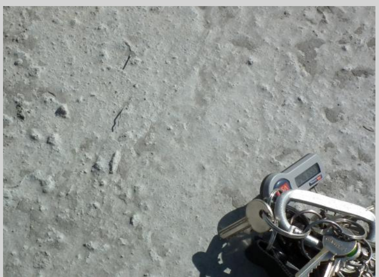
Figure 8.11. The surface appearance of SFRSCC after manual trowelling. No other surface finishing procedures have been applied. Difficult to submerge all the fibres.
