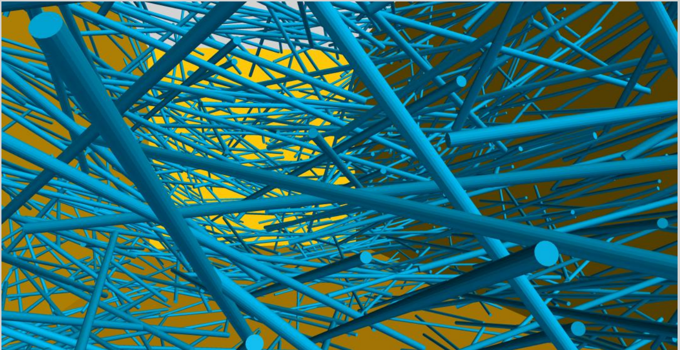
Figure 7.16: Picture to illustrate the individual fibres included in the simulation of a standard beam cast with SFRSCC.
