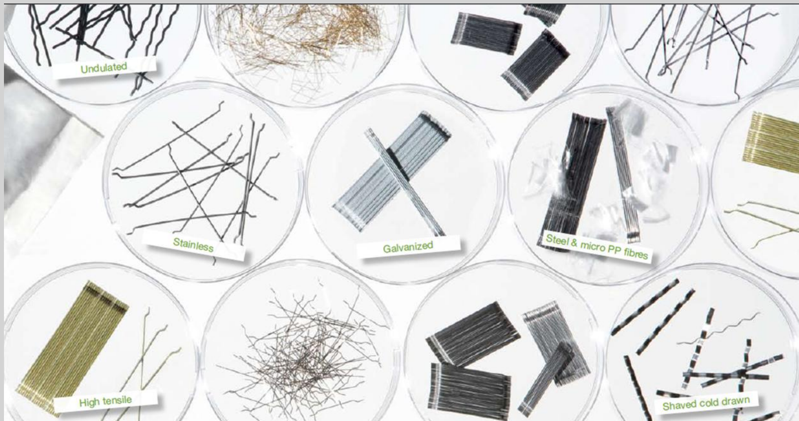
Figure 2.2: Examples of different types of steel fibres.
