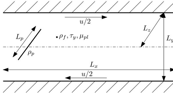
Figure 4: Couette flow geometry.
