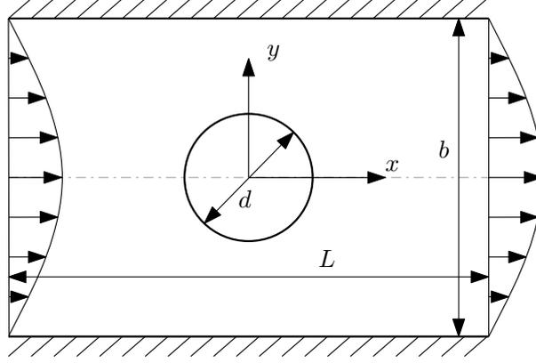
Figure 2: Geometry of the Poiseuille flow model
